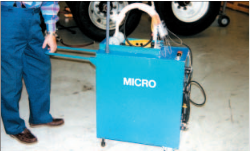
Photo 1 - The Micro Tire Tester is a very portable unit with a fold down handle and two rollers, allowing it to be easily moved from one spreader to another in just a few seconds.
