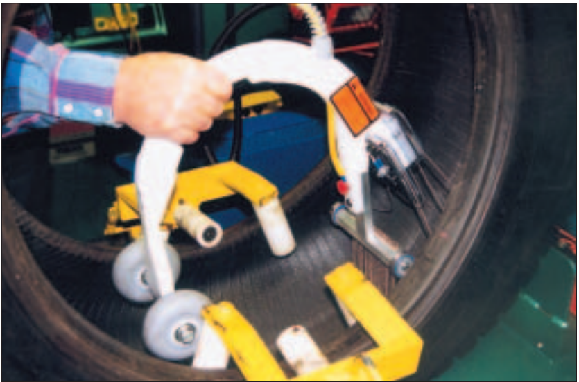
Photo IV - The Micro scanner is very lightweight (4.5 lbs) and can quickly and easily move in and out of a tire with one hand.
